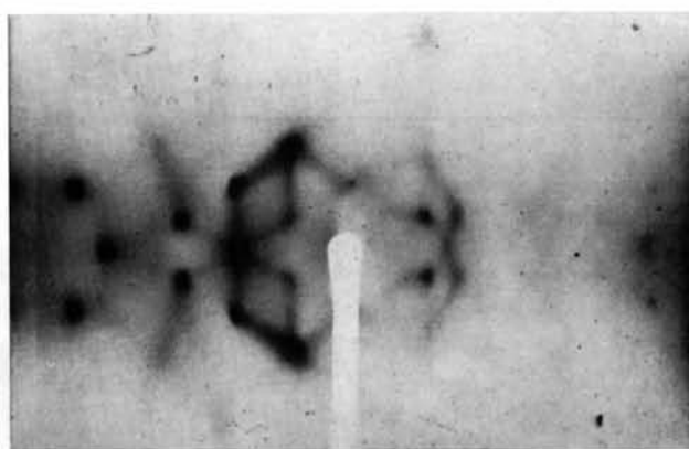
Fig. 3. Monochromatic \text{Cu } K\alpha radiation 28^\circ from c axis, [1\bar{1}\dagger 0] vertical. Exposure 4 hr.; -5^\circ\text{C} . The rounded diffuse spots at the intersections of narrow streaks are well shown.
